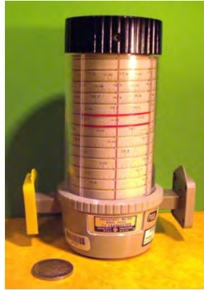
Figure 21.15: An absorption wave meter can be used to measure the frequency of microwave (courtesy of Wiki [120]).
